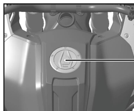
Spare fuel tank capacity 2.0L
