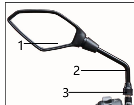
The fastening torque for nut 3:40Nm
